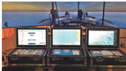
Figure 2 Ship bridge simulator environment studying safe navigation (c.f. also [13])
