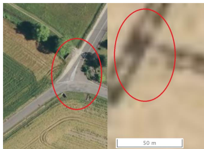
Fig. 25: A superimposed French staff plan with a paneled view shows a positioning error of an old crossroads of more than 50 meters. In addition, the plan on the right shows a rather large pixelation when the zoom is high, which hinders precision work.
