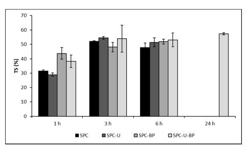
Figure 5. Thickness swelling (TS) of the injection-molded pieces after immersion in water.
