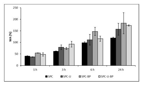
Figure 6. Water absorption (WA) of the injection-molded pieces after immersion in water.
