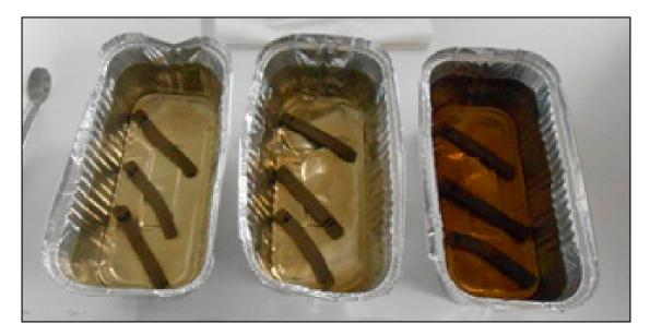
**Figure 7.** Macroscopical image illustrating the change of the visual of the SPC injection-molded piece-water system upon increasing the solid–liquid contact time (from left to right, 1, 3, and 6 h).
