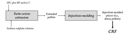
Figure 2. Schematic diagram of the process developed for the preparation of the fertilizers.
