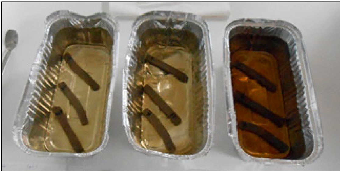
Figure 7. Macroscopic image illustrating the change of the visual of the SPC injection-molded piece–water system upon increasing the solid–liquid contact time (from left to right, 1, 3, and 6 h).
