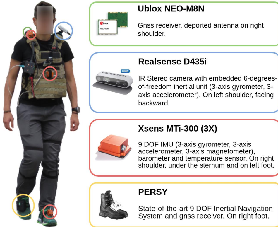
Fig. 1. Test setup for the acquisition of the data for the indoor competition challenge MALIN
