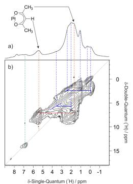
Fig. 3 a) <sup>1</sup>H MAS NMR and b) <sup>1</sup>H-<sup>1</sup>H DQ-SQ MAS NMR spectra (800 MHz, spinning speed 20 kHz); Red lines : signals related to Pt-acac; Blue lines : signals related to alumina hydroxyls; Green lines : signals related to olefinic by-products.
