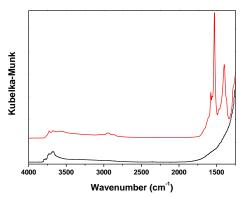
Fig. 1 DRIFT spectrum of  $Pt(acac)_2$  after reaction with  $\gamma$ -Al<sub>2</sub>O<sub>3</sub> in toluene at room temperature.
