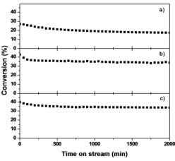
**Fig. 5** Conversion of DMBH on a) Pt/Al<sub>2</sub>O<sub>3</sub>; b) Pt/Li-Al<sub>2</sub>O<sub>3</sub>; and c) PtSn/Li-Al<sub>2</sub>O<sub>3</sub>. 200 mg, P<sub>DMBH</sub> = 350 mbar, 10 ccm of H<sub>2</sub>, 500 °C <sup>25</sup> propene and ethane (See Table S1). The formation of
