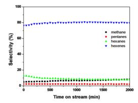
Fig. 6 Time-resolved evolution of the selectivity of products on PtSn/Li-Al<sub>2</sub>O<sub>3</sub>, 200 mg,  $P_{DMBH} = 350$  mbar, 10 ccm of H<sub>2</sub>, 500 °C. Traces (< 1%) have been omitted for clarity.
