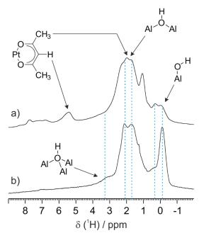
Fig. 2 <sup>1</sup>H MAS NMR spectrum of a)  $Pt(acac)_2$  supported on alumina and b)  $\gamma$ -Al<sub>2</sub>O<sub>3-500</sub> (800 MHz, spinning speed 20 kHz).
