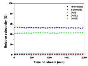
Fig. 7 Time-resolved evolution of relative selectivity of acyclic C6 on PtSn/Li-Al<sub>2</sub>O<sub>3</sub>, 200mg,  $P_{DMBH} = 350$  mbar, 10ccm of H<sub>2</sub>, 500°C.
