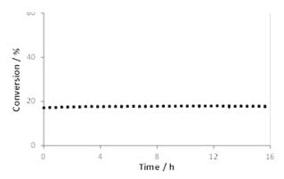
**Fig. 8** Conversion of 2,3-DMBH on PtSn/Li-Al<sub>2</sub>O<sub>3</sub>, 100mg, saturation pressure, 5ccm of N<sub>2</sub>, 390°C.
