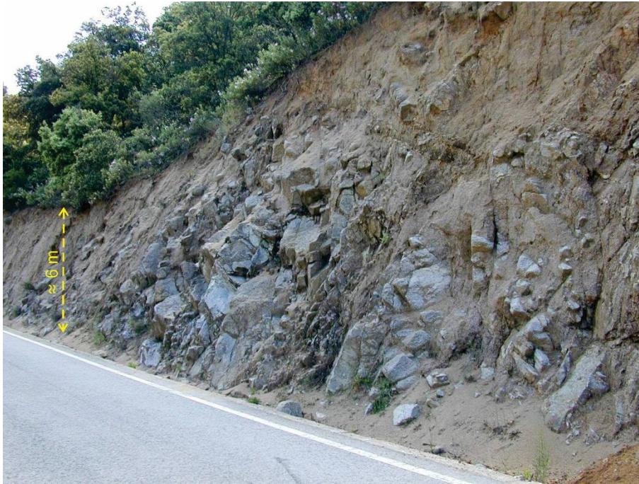
Fig. 1 Exposure of physically and chemically weathered granodiorite (an intrusive, igneous rock comparable to granite); zones of fresh, hard, and strong granodiorite (bluish-grey colored) occur in between zones of granodiorite fallen apart in smaller blocks and zones completely decomposed into loose soil material (brownish colored). Note the general increase of decay upwards to the original topographical surface (vegetated) (Road T710, Falset - Gratallops, Catalunya, Spain; photo courtesy of W. Verwaal 2002)
