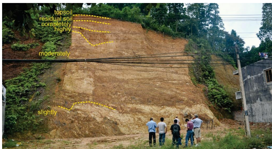
Fig. 6 Weathered cut slope in gneiss and schist in a tropical climate (Weathering grades follow Table 2 for rock masses) (Yên Bái City, Vietnam; photo courtesy D. Alkema, 2010)
