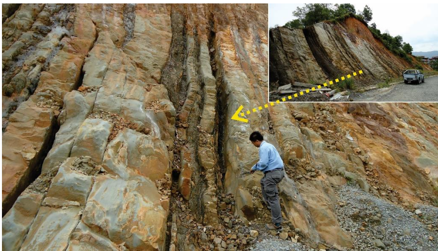
Fig. 7 Different lithologies with different susceptibility to weathering result in groundmasses with layers with different states of weathering. The grey, light-brown sandstone is more resistant to weathering than the dark-brown, black shale that is already completely weathered and partially eroded within five years after excavation giving the inserts in the groundmass (Flysch deposit of sandstone layers mainly consisting of quartz grains, alternating with shale; Kota Kinabalu, Malaysia, 2011)
