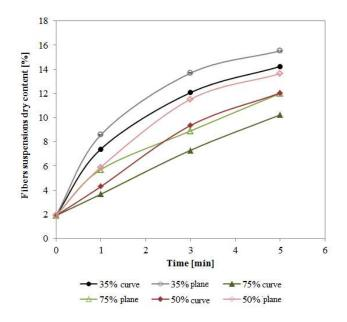
Figure 6. Evacuation of water of the cellulose fiber suspension by aspiration using the different printed molds for the plane part and the curve part of the mold.
