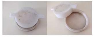
Figure 9. Mold produced by 3D printing with a filling degree of 35% to produce 2D cellulosic object.
