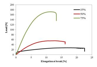
Figure 5. Mechanical resistance of 3D printed objects depending on their filling degree.
