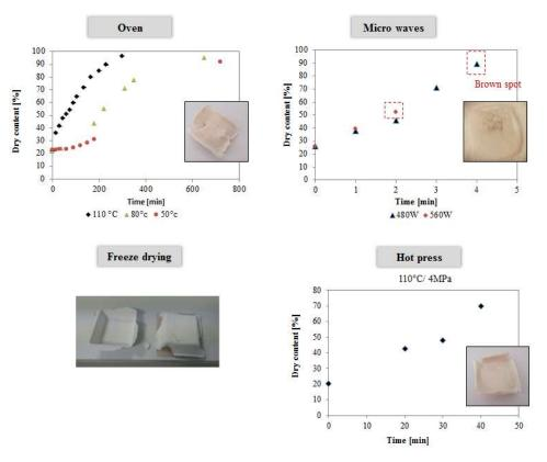
Figure 8. Different methods used to dry the nanocellulosic mats made in the 3D printed mold.
