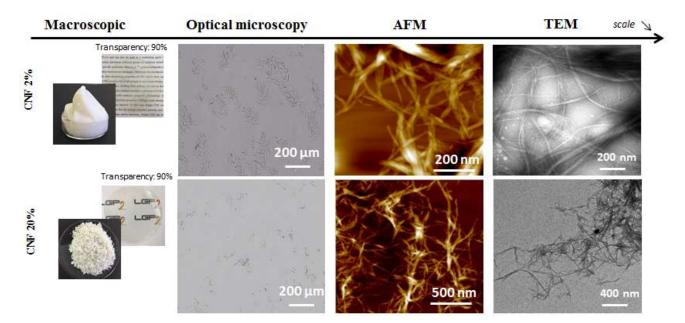
Figure 2. Characterizations of CNF produced by TSE.
