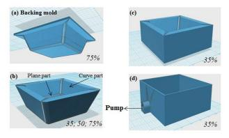
Figure 3. 3D printed mold designed on four parts to simulate the cellulose molding process.
