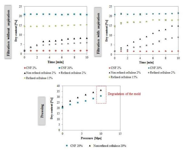
**Figure 7.** Dry content of the CNF mat formed in the mold plane part filtration (step 1) and pressing (step 2).
