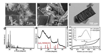
Figure 1. SEM images of the Al-MOF (a) and  $Al_2O_3@MOF$ -C (b) and the TEM images of the  $Al_2O_3@MOF$ -C (c). XRD patterns of the Al-MOF (d) and  $Al_2O_3@MOF$ -C (e) and the  $N_2$  adsorption/desorption isotherms of  $Al_2O_3@MOF$ -C (f) and corresponding pore distribution curves (inserted figure in f).
