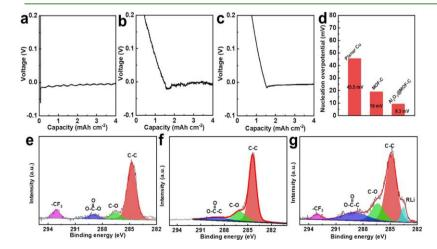
Figure 3. Voltage-capacity curves of the Li deposits on different substrates: (a) planar Cu, (b) MOF-C, and (c) Al<sub>2</sub>O<sub>3</sub>@MOF-C. Nucleation overpotential on different substrates at 0.2 mA cm<sup>-2</sup>(d). XPS of C 1s spectra recorded for: (e) the Cu@Li (0.5 mAh cm<sup>-2</sup>), (f) pristine Al<sub>2</sub>O<sub>3</sub>@ MOF-C, and (g) Al<sub>2</sub>O<sub>3</sub>@MOF-C after plating 0.5 mAh cm<sup>-2</sup>Li.
