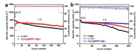
$Figure\ 6.\ Cycling\ performances\ of\ the\ (a)\ Li-S\ and\ (b)\ Li/LiFePO_4\ cells\ using\ different\ Li-metal\ anodes.$
