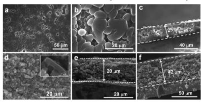
Figure 2. Top-view SEM images of the Cu@Li (a, b),  $Al_2O_3@MOF-C@Li$  electrodes (d) and the high-resolution image of  $Al_2O_3@MOF-C@Li$  (inserted figure in d). The side-view SEM images of Cu@Li (c),  $Al_2O_3@MOF-C$  (e), and  $Al_2O_3@MOF-C@Li$  (f) electrodes after plating 6 mAh cm<sup>-2</sup> of Li at a current density of 1 mA cm<sup>-2</sup>.
