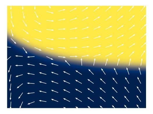
Figure 3: Zoomed-in view of the meniscus formed by PEG 3350 for a high wall velocity (Ca =  $4.6 \cdot 10^{-3}$ ,  $V = 70 \,\mathrm{mm/min}$ ). The area shown here is approximately 7 mm by 4 mm. The velocity field shown here is not proportional.
