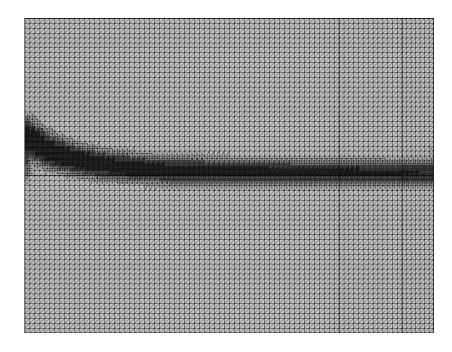
Figure X: Refined mesh obtained with a low plate velocity in a PEG 3350. The mesh displayed here contains 28563 elements, with sizes ranging from 40 to  $160\,\mu m$ . The PEG 3350 occupies the bottom part of the domain.
