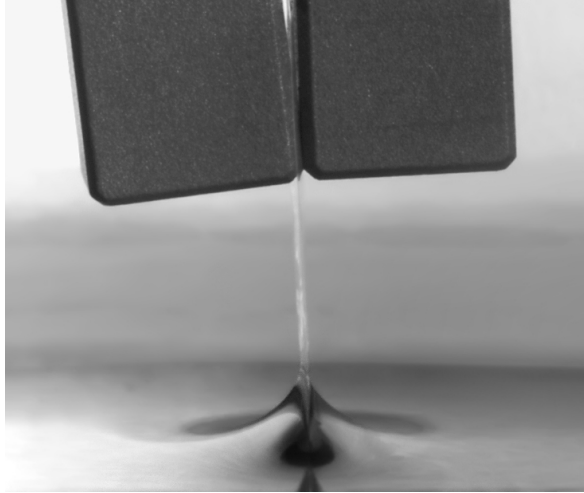
Figure V: Snapshot of the meniscus formed by PEG 3350 on a static cellulosic substrate, captured at an angle above the liquid surface. The substrate is attached to a microbalance, measuring the force exerted by the contact line. This allows to evaluate the macroscopic contact angle.
