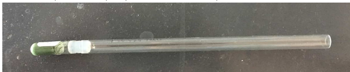
Figure 6 : picture of the sample NMR tube with its extension for introduction in the relaxometers.
