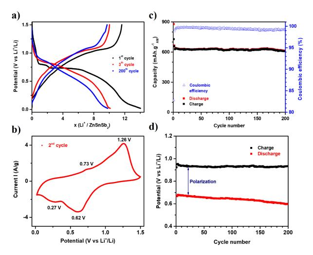
Figure 2: Galvanostatic profile a) and cyclic voltammetry b) of ZnSnSb<sub>2</sub> cycled between 0.02 and 1.5 V vs Li<sup>+</sup>/Li. Specific capacity and coulombic efficiency c), average discharge/charge potentials d) as function of cycle number.
