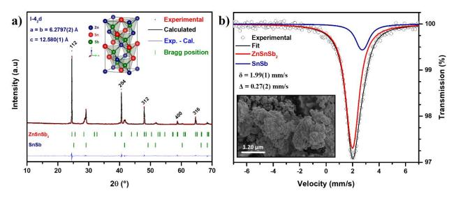
Figure 1: XRD pattern with the tetragonal chalcopyrite structure representation a), and <sup>119</sup>Sn Mössbauer spectrum at 25K with SEM picture b), of ZnSnSb<sub>2</sub> powder.
