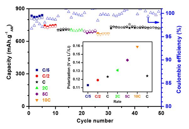
*Figure 3: Rate capability and polarization (inset) of* ZnSnSb<sub>2</sub> *cycled at various current from* C/5 *to* 10C *between* 0.02 *to* 1.5 V *vs* Li<sup>+</sup>/Li *at room temperature. (Filled: discharge; empty: charge).*
