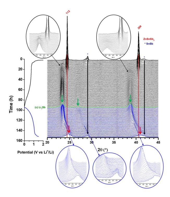
*Figure 4: Operando XRD patterns collected during the first cycle of* ZnSnSb<sub>2</sub> *cycled between 0.02 to 1.5 V vs* Li<sup>+</sup>/Li at a C/5 rate at room temperature. Black and blue lines correspond to the first discharge and charge respectively. The green diffractogram represents the end of the discharge.
