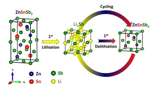
Figure 5: Electrochemical mechanism proposed for ZnSnSb<sub>2</sub> anode in Li-ion batteries.
