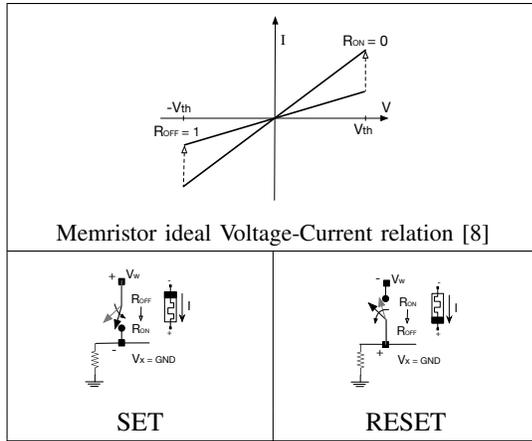
Figure 1. Set and Reset operations [14]
