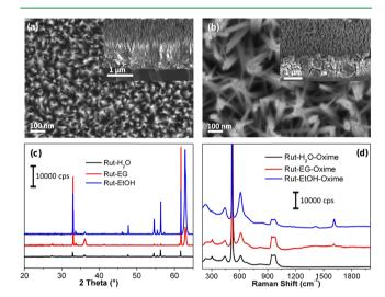
Figure 5. Top and cross-sectional (inset) SEM images of rutile TiO<sub>2</sub> NRs prepared by replacing ethanol with (a) ethylene glycol and (b) water in the presence of hydrochloric acid and 0.25 mL of TTIP at 150 °C for 8 h. (c) XRD of the nanostructure prepared with water, ethylene glycol, and ethanol. (d) Raman spectra of the three different nanostructures functionalized with oxime molecules.
