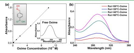
Figure 4. (a) UV-vis oxime calibration curve and UV-vis absorption spectrum of the free oxime molecule in NaOH solution (pH 12). Inset shows the scheme of the oxime molecule (the green part is the tethering site for the TiO<sub>2</sub> nanostructure, and the red one is the oxime function). (b) UV-vis spectra of desorbed oxime anchored on each rutile TiO<sub>2</sub> nanorod surface.
