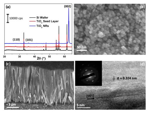
Figure 1. (a) XRD patterns of the as-prepared TiO2 NR film (blue), TiO2 seed layer made by sputtering (red), and a silicon wafer substrate as a reference (black). (b, c) SEM images of a vertically oriented rutile TiO2 nanorod film grown on a silicon wafer surface prepared in solvothermal conditions with 0.5 mL of TTIP, 15 mL of HCl, 15 mL of ETOH, 0.5 mL triethylamine hydrochloride (TEACl) at 150 °C for 8 h, (d) TEM image of a single rutile TiO2 nanorod.
