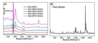
Figure 3. (a) Raman spectra of rutile nanorods synthesized at different growth temperatures and functionalized with oxime. (b) Raman spectra of free oxime molecules used for anchoring on each rutile TiO2 nanorod surface.
