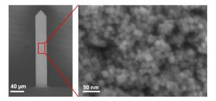
**Figure 8.**  ${\rm TiO_2}$  nanostructured cantilever prepared in ethanol, hydrochloric acid, 0.5 mL of TEACl, and 0.5 mL of TTIP at 150  $^{\circ}{\rm C}$  for 8 h.
