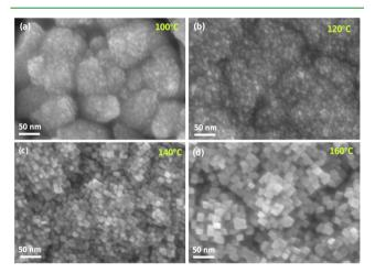
Figure 2. Top-surface SEM images of rutile TiO2 films grown at different synthesis temperatures: (a) 100 °C, (b)120 °C, (c)140 °C, and (d) 160 °C (keeping the other parameters constant).
