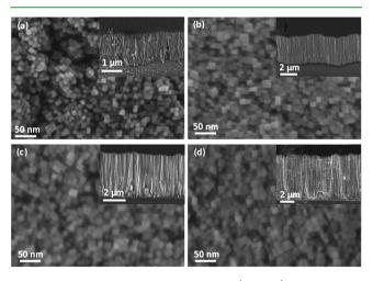
Figure 6. Top- and side-view SEM images (in inset) of rutile TiO2 NR films grown at 150 °C for 8 h with different volumes of TTIP in a mixture (1:1) of hydrochloric acid and ethanol: (a) 0.25 mL, (b) 1 mL, (c) 2 mL, and (d) 3 mL.
