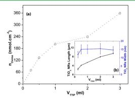
Figure 7. (a) Oxime loading onto TiO2 nanorods synthesized at different TTIP volumes. (b) Influence of the TTIP volume on the length and the diameter of the nanorods.
