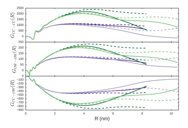
FIG. 8: KB integrals,  $G_{ij}(R)$ , at  $x_t = 0.06$  as functions of R obtained from NVT (green lines) and NPT (purple lines) simulations with 128000 (dark lines) or 256000 (light lines) particles. The solid and dashed line represented results without and with estimated finite-size corrections to the pair correlation functions, respectively.
