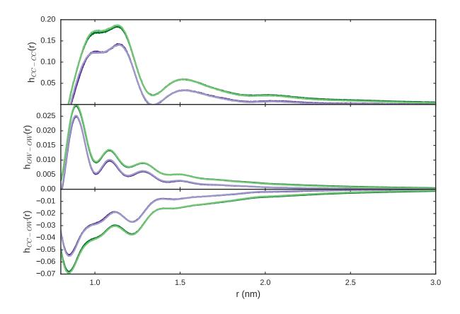
FIG. 7: Pair correlation functions  $[h_{ij}(r) = g_{ij}(r) - 1]$  at  $x_t = 0.06 \ (\sim 1 - 3 \text{ nm})$ , from NVT (green lines) and NPT (purple lines) simulations with 128000 (dark lines) or 256000 (light lines) particles. Results are shown for i = j = CC (top panel), the i = j = OW (middle panel) and i = CC, j = OW (bottom panel).
