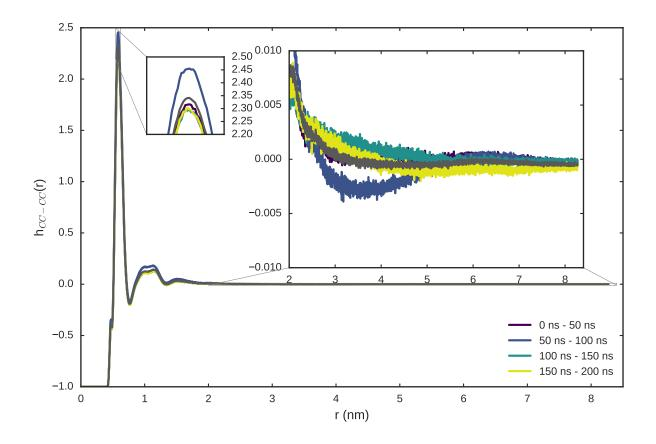
FIG. 5: TBA-TBA pair correlation functions at  $x_t = 0.06$  from 50 ns simulations blocks of a 200 ns *NPT* simulation with 128000 particles. The average over the full 200 ns is shown in grey.
