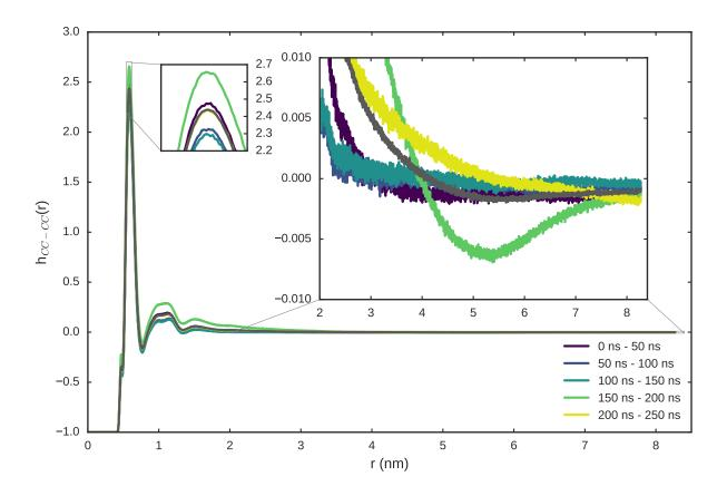
FIG. 4: TBA-TBA pair correlation functions  $[h_{CC-CC}(r) = g_{CC-CC}(r) - 1]$  at  $x_t = 0.06$  from 50 ns simulations blocks of a 250 ns NVT simulation with 128000 particles. The average over the full 250 ns is shown in grey.
