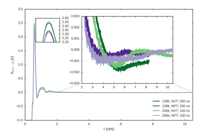
FIG. 6: TBA-TBA pair correlation functions at  $x_t = 0.06$  from NVT (green lines) and NPT (purple lines) simulations with 128000 (dark lines) or 256000 (light lines) particles. Simulation times for the 128000-particle systems are 250 ns (NVT) and 200 ns (NPT), and for the 256000-particle systems are 100 ns (both NVT and NPT).
