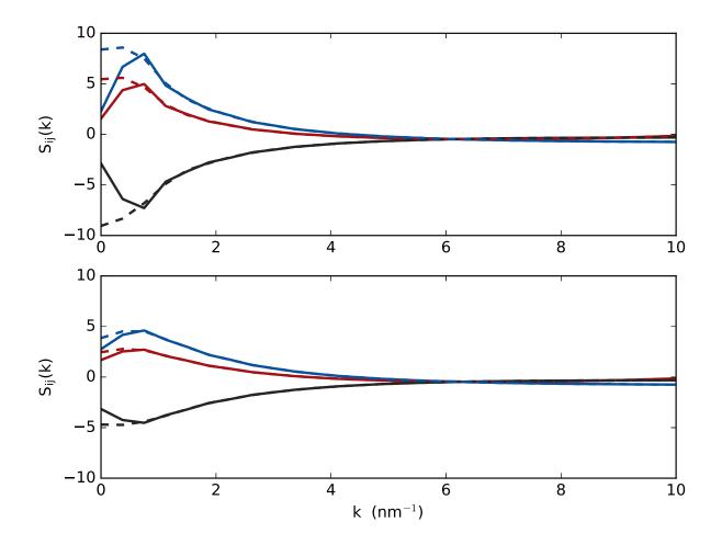
FIG. 9: Partial structure factors at  $x_t = 0.06$ ,  $S_{CC-CC}(k)$  (red),  $S_{CC-OW}(k)$  (black) and  $S_{OW-OW}(k)$  (blue), from 100 ns NVT (top) and NPT (bottom) simulations with 128000 particles. Results obtained both with and without estimated finite-size corrections to the pair correlations are shown as dashed and solid lines, respectively.
