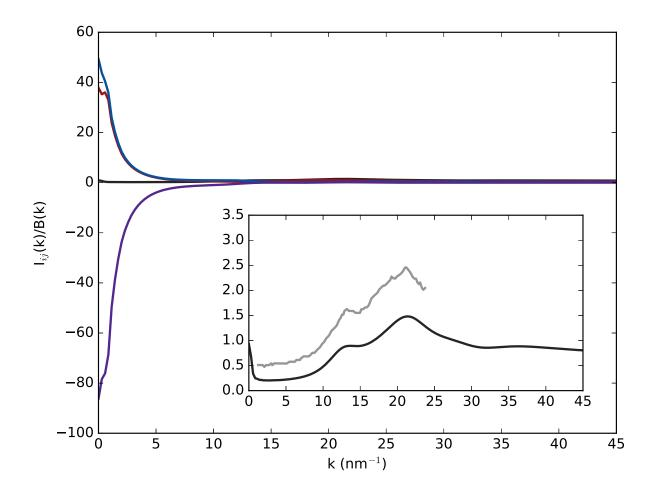
FIG. 11: SANS scattering functions at  $x_t = 0.1$ . The results shown are averages over three independent *NPT* simulations (250 ns in total) employing 256000 molecules. Partial structure factors for TBA-TBA (red), water-water (blue), and TBA-water (purple) are shown. The deuterium scattering length was used for all hydrogen atoms. The total scattering from simulations (black) is compared with experimental results<sup>23</sup> (grey) in the inset.
