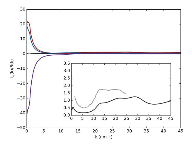
FIG. 12: SAXS scattering functions at  $x_t = 0.1$ . The results shown are averages over three independent *NPT* simulations (250 ns in total) employing 256000 molecules. Partial structure factors for TBA-TBA (red), water-water (blue), and TBA-water (purple) are shown. The deuterium scattering length was used for all hydrogen atoms. The total scattering from simulations (black) is compared with experimental results<sup>23</sup> (grey) in the inset.
