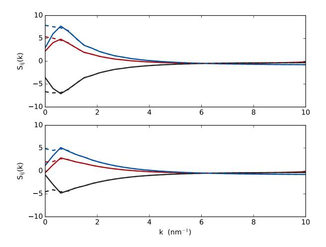
FIG. 10: Partial structure factors at  $x_t = 0.06$ ,  $S_{CC-CC}(k)$  (red),  $S_{CC-OW}(k)$  (black) and  $S_{OW-OW}(k)$  (blue), from 100 ns NVT (top) and NPT (bottom) simulations with 256000 particles. Results obtained both with and without estimated finite-size corrections to the pair correlation functions are shown as dashed and solid lines, respectively.
