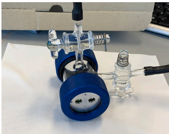
Figure S1. Gas cell featuring a custom metal lid with two orifices where the samples are placed and fixed.
