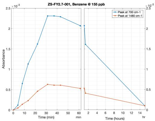
**Figure S7**: Kinetic response to a 155 ppb benzene (1-30 min) and flushing in dry nitrogen (30 min -15h) to show the reversibility at room temperature.
