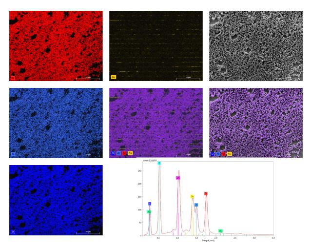
Figure S4: Elemental compositions mapping for a FAU coating on nanoantennas and EDX analysis
