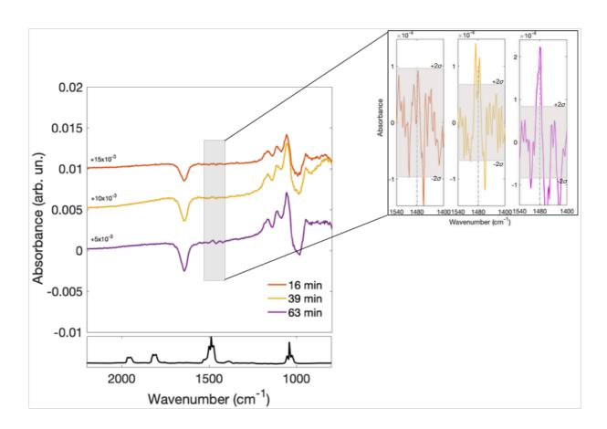
**Figure S8**: IR spectra corresponding to Figure 5c for perpendicular polarisation (exposure to 25ppb of benzene)
