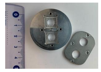
Figure S1. Gas cell featuring a custom metal lid with two orifices where the samples are placed and fixed.
