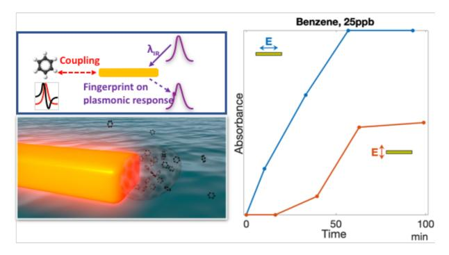
The concerted action of infrared resonant nano-antennas with an ultra-thin zeolite concentrating coating, enables unprecedented rapid detection of benzene traces (25 ppb). In this hybrid material, the zeolite coating effectively traps VOCs analytes nearby the hotspots of nano-antennas, thus enabling Surface Enhanced Infrared Absorption (SEIRA). Sensitivity equivalent to a ~120 m long optical path is achieved in a ~200 nm layer.
