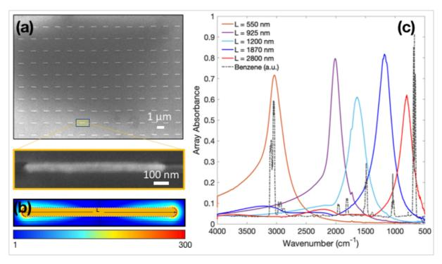
**Figure 3**: (a) SEM image of a resonant nano-antenna array composed of phased gold nanorods. (b) Field distribution at resonance, normalized by the incident field. (c) IR spectra of nanoantenna array of different length overlapped with benzene spectrum (dotted spectrum).
