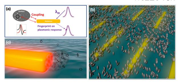
**Figure 1:** (a) Surface-Enhanced Infrared Absorption (SEIRA) concept: near-field coupling between molecular/phonon transitions and optical resonances enables the amplification of the fingerprint. (b) Gold nanorods array coated by zeolite nanocrystals able to trap benzene in regions where the near field enhancement is the highest (c).
