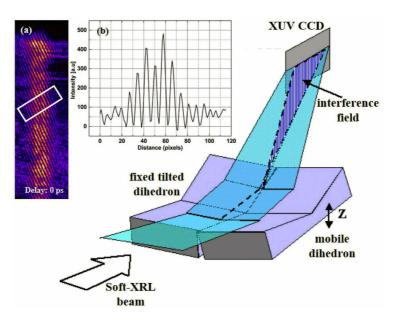
**Fig. 5.** Principle of wavefront-division variable path-difference interferometer comprising a dihedron pair. The hatched area represents the interference field. Inset figure (a) depicts a raw interferogram corresponding to a null delay for grazing incidence pumping angle of  $32^{\circ}$  and  $T_{IR} = 4ps$ . Line representation of the interferogram extracted from the region enclosed within the box (inset (a)) is presented in (b).
