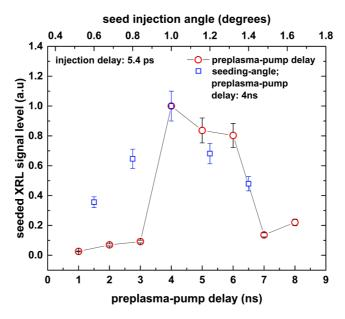
**Fig. 6.** Normalized seeded-XRL intensity as a function of delay between preplasma and pump pulse; high-harmonic seed is injected 5.4ps after the intensity peak of pump. For the given delay, most efficient amplification was observed for seeding angle of  $1^{\circ}$ .
