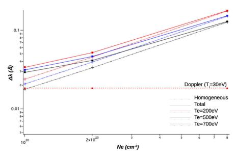
**Fig. 7.** Intrinsic linewidth (FWHM) of Ne-like Ti soft-XRL line as a function of the electron density  $N_e$  for three levels of electron temperature  $T_e$ .
