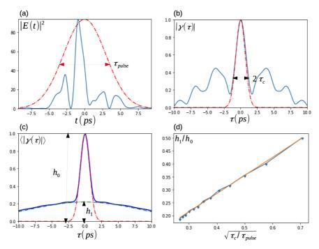
**Fig. 8.** ASE X-ray laser pulse modelling. (a) single-pulse temporal profile. Simulation of the modulus of its first-order autocorrelation function for (b) a single pulse (c) averaged over N=100 pulses. Fitting curves showed in red and green are presented in the main text. (d) The relationship between the different fitting parameters.
