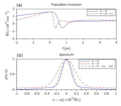
**Fig. 9.** Bloch-Maxwell simulation of the XRL seeded operation for  $\Phi = 22^{\circ}$ ,  $T_{IR} = 7ps$  and  $\Phi = 32^{\circ}$ ,  $T_{IR} = 4ps$ . (a) shows population inversion under aforementioned conditions. The simulated spectra of the seeded XRL for both configurations, along with the ASE-XRL spectrum obtained from experimental coherence measurement for  $\Phi = 22^{\circ}$ ,  $T_{IR} = 7ps$  is presented in (b) by dashed-black curve.
