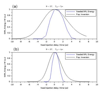
**Fig. 10.** Bloch-Maxwell simulation of the XRL seeded output energy for different seed injection delays (blue curves) for input parameters corresponding to  $\Phi = 22^{\circ}$ ,  $T_{IR} = 7ps$  (a) and  $\Phi = 32^{\circ}$ ,  $T_{IR} = 4ps$  (b). Evolution of the population inversion in the absence of laser field is plotted in black.
