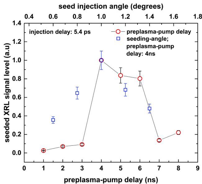
**Fig. 6.** Normalized seeded-XRL intensity as a function of delay between preplasma and pump pulse; high-harmonic seed is injected  $5.4\text{ps}$  after the intensity peak of pump. For the given delay, most efficient amplification was observed for seeding angle of  $1^\circ$ .
