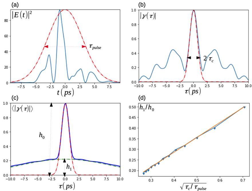
**Fig. 8.** ASE X-ray laser pulse modelling. (a) single-pulse temporal profile. Simulation of the modulus of its first-order autocorrelation function for (b) a single pulse (c) averaged over  $N=100$  pulses. Fitting curves showed in red and green are presented in the main text. (d) The relationship between the different fitting parameters.
