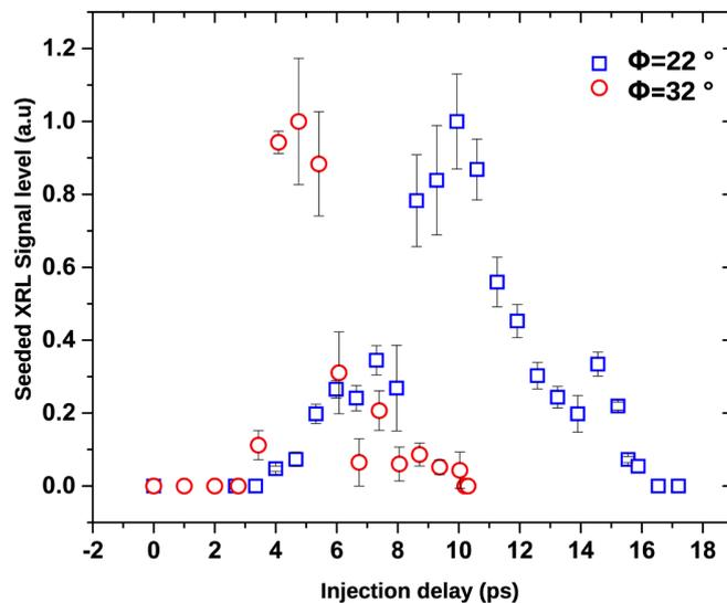
**Fig. 3.** Normalized seeded-XRL energy as a function of injection delays for low ( $\Phi = 22^\circ$  and  $T_{IR} = 7ps$ ) and high ( $\Phi = 32^\circ$  and  $T_{IR} = 4ps$ ) electron density amplifiers. In the high-density scenario, XRL plasma was seeded at an off-axis injection angle of  $\sim 1^\circ$  to counter the effects of refraction (see Appendix C). For both the configurations, the IR pump was delayed by 4ns with respect to the peak of preplasma forming pulse.
