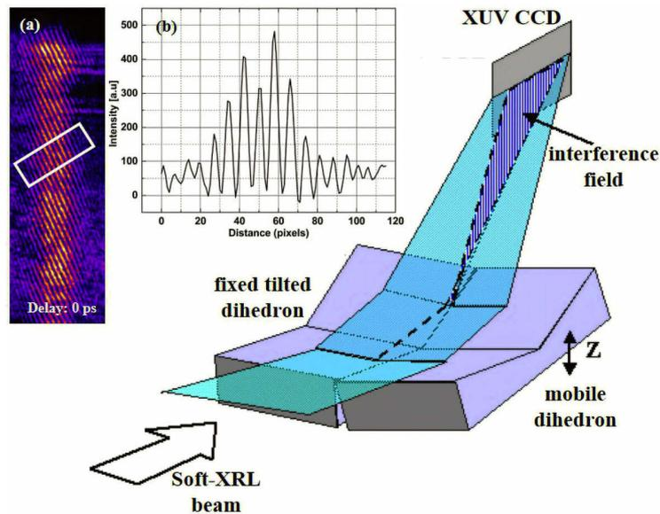
**Fig. 5.** Principle of wavefront-division variable path-difference interferometer comprising a dihedron pair. The hatched area represents the interference field. Inset figure (a) depicts a raw interferogram corresponding to a null delay for grazing incidence pumping angle of  $32^\circ$  and  $T_{IR} = 4ps$ . Line representation of the interferogram extracted from the region enclosed within the box (inset (a)) is presented in (b).
