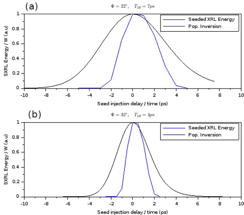
**Fig. 10.** Bloch-Maxwell simulation of the XRL seeded output energy for different seed injection delays (blue curves) for input parameters corresponding to  $\Phi = 22^\circ, T_{IR} = 7 ps$  (a) and  $\Phi = 32^\circ, T_{IR} = 4 ps$  (b). Evolution of the population inversion in the absence of laser field is plotted in black.
