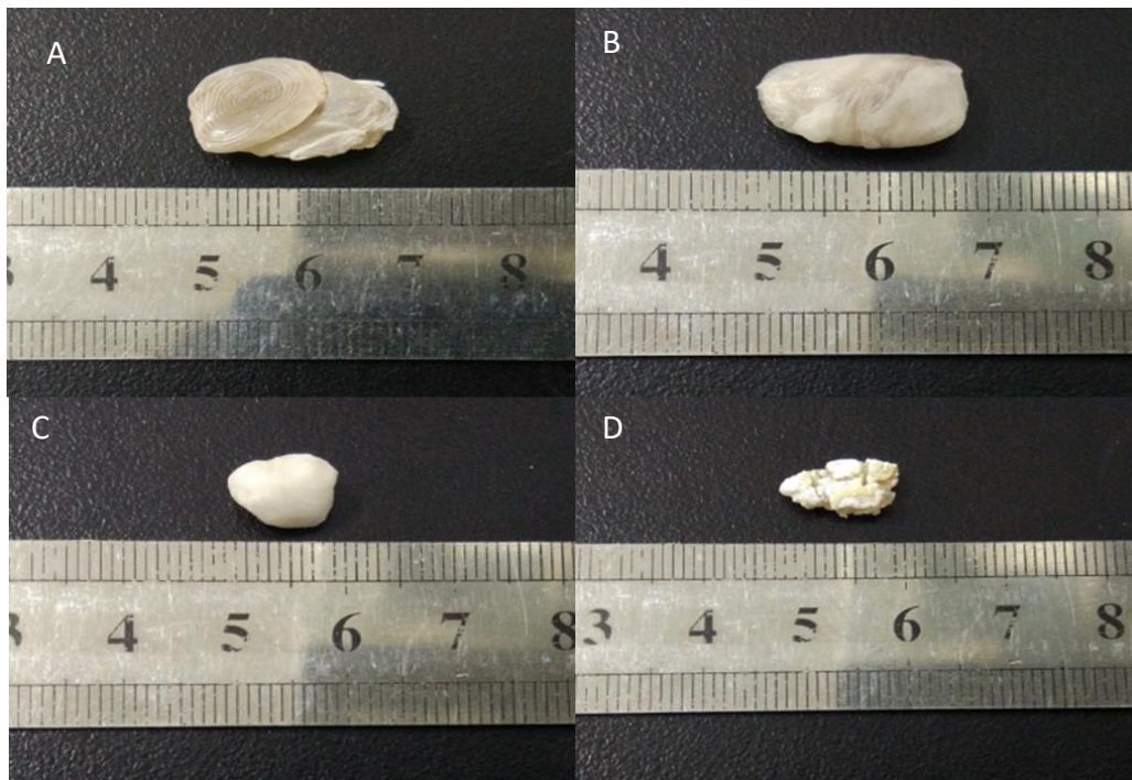
Figure 8. Shape changes during in vivo degradation of the occluders: (A) 10 days; (B) 30 days; (C) 60 days; (D) 90 days.
