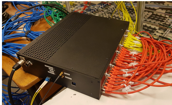
Figure 2: Photograph of the acoustic data acquisition system. The colored cables are RJ45 linking the buffer cards to acquisition system.
