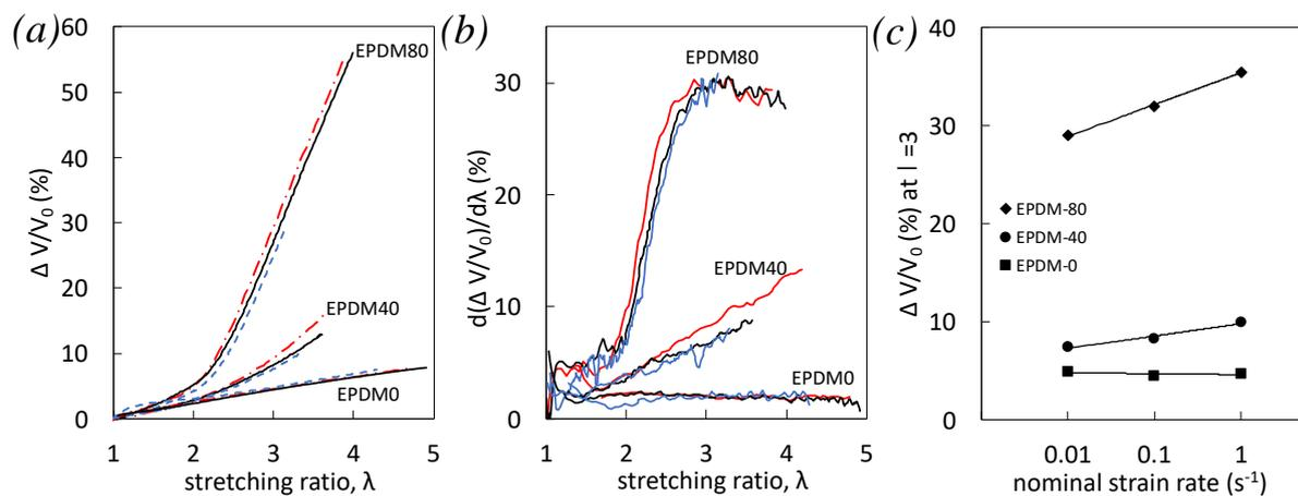
**Figure 3.** Volumetric strain (a) and rate of volumetric strain (b) versus strain for EPDM-0, EPDM-40 and EPDM-80 during single uniaxial loading at the nominal strain rates  $10^{-2} \cdot s^{-1}$  (blue dotted line),  $10^{-1} \cdot s^{-1}$  (black continuous line), and  $1 \cdot s^{-1}$  (red dashed dotted line), (c) Volumetric strain at  $\lambda=3$  versus nominal strain rate for EPDM-0, EPDM-40 and EPDM-80.
