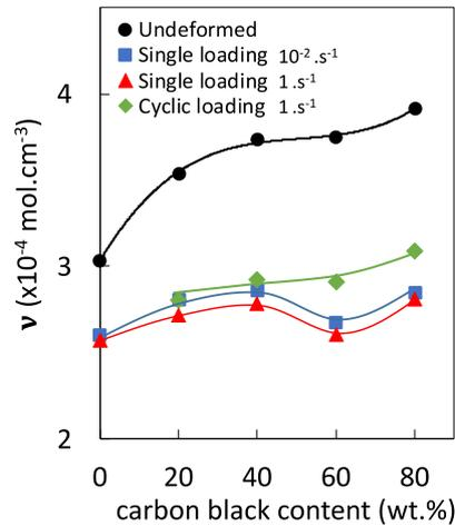
**Figure 1.** Average network chain densities of EPDM with filler content of 0, 20, 40, 60 and 80 phr for untested (undeformed) specimen (ring symbols), for cyclically loaded specimen at the nominal strain rate  $1 \text{ s}^{-1}$  (diamond symbols), for single loaded specimens at the nominal strain rate  $10^{-2} \text{ s}^{-1}$  (square symbols) and for single loaded specimens at the nominal strain rate  $1 \text{ s}^{-1}$  (square symbols).
