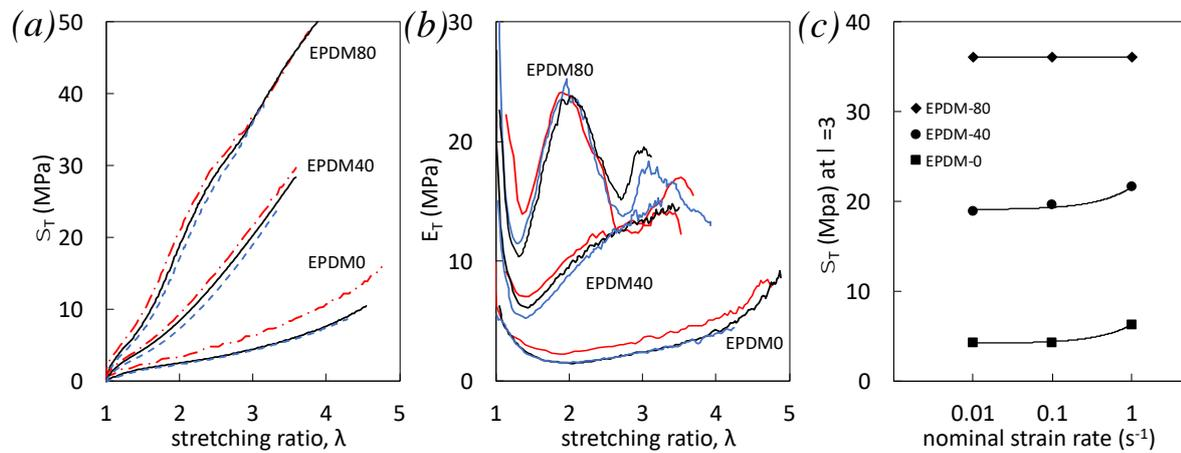
**Figure 2.** True stress (a), tangent modulus (b) versus strain for EPDM-0, EPDM-40 and EPDM-80 during single uniaxial loading at the nominal strain rates  $10^{-2} \text{ s}^{-1}$  (blue dotted line),  $10^{-1} \text{ s}^{-1}$  (black continuous line), and  $1 \text{ s}^{-1}$  (red dashed dotted line), (c) True stress at  $\lambda=3$  versus nominal strain rate for EPDM-0, EPDM-40 and EPDM-80.
