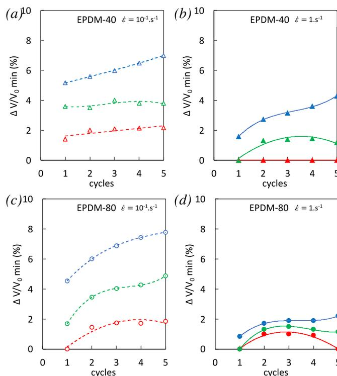
**Figure 9.** Minimum volumetric strain reached during multiple cyclic loadings performed at three different stretching ratios  $\lambda_1 = 2$  (in red),  $\lambda_2 = 2.9$  (in green) and  $\lambda_3 = 3.7$  (in blue) and for the strain rates  $10^{-1} \text{ s}^{-1}$  (unfilled symbols) and  $1 \text{ s}^{-1}$  (filled symbols) for EPDM-40 (a) and EPDM-80 (b).
