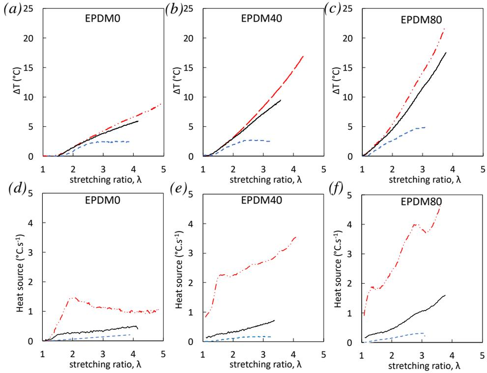
**Figure 4.** Self-heating versus strain for EPDM-0 (a), EPDM-40 (b) and EPDM-80 (c) during single uniaxial loading at the nominal strain rates  $10^{-2} \cdot \text{s}^{-1}$  (blue dotted line),  $10^{-1} \cdot \text{s}^{-1}$  (black continuous line), and  $1 \cdot \text{s}^{-1}$  (red dashed dotted line). Corresponding heat source versus strain for EPDM-0 (d), EPDM-40 (e) and EPDM-80 (f).
