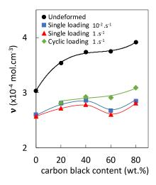
**Figure 1.** Average network chain densities of EPDM with filler content of 0, 20, 40, 60 and 80 phr for untested (undeformed) specimen (ring symbols), for cyclically loaded specimen at the nominal strain rate 1  $\cdot$ s<sup>-1</sup> (diamond symbols), for single loaded specimens at the nominal strain rate  $10^{-2}$  s.<sup>-1</sup> (square symbols) and for single loaded specimens at the nominal strain rate 1  $\cdot$ s<sup>-1</sup> (square symbols).
