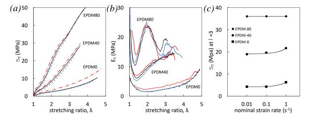
**Figure 2.** True stress (*a*), tangent modulus (*b*) versus strain for EPDM-0, EPDM-40 and EPDM-80 during single uniaxial loading at the nominal strain rates  $10^{-2}$  .s<sup>-1</sup> (blue dotted line),  $10^{-1}$  .s<sup>-1</sup> (black continuous line), and 1 .s<sup>-1</sup> (red dashed dotted line), (*c*) True stress at  $\lambda$ =3 versus nominal strain rate for EPDM-0, EPDM-40 and EPDM-80.
