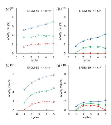
**Figure 9.** Minimum volumetric strain reached during multiple cyclic loadings performed at three different stretching ratios  $\lambda_1 = 2$  (in red),  $\lambda_2 = 2.9$  (in green) and  $\lambda_3 = 3.7$  (in blue) and for the strain rates  $10^{-1} \cdot \text{s}^{-1}$  (unfilled symbols) and  $1 \cdot \text{s}^{-1}$  (filled symbols) for EPDM-40 (a) and EPDM-80 (b).
