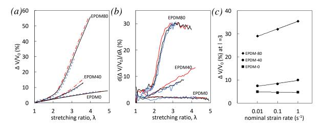
**Figure 3.** Volumetric strain (*a*) and rate of volumetric strain (*b*) versus strain for EPDM-0, EPDM-40 and EPDM-80 during single uniaxial loading at the nominal strain rates  $10^{-2}$ .s<sup>-1</sup>(blue dotted line),  $10^{-1}$ .s<sup>-1</sup> (black continuous line), and 1.s<sup>-1</sup> (red dashed dotted line), (*c*) Volumetric strain at  $\lambda$ =3 versus nominal strain rate for EPDM-0, EPDM-40 and EPDM-80.
