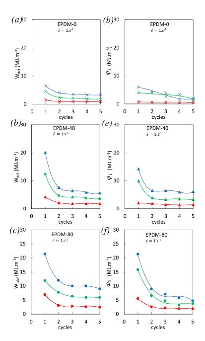
**Figure 6.** Deformation energy estimated from the area under the stress strain curve (equation 7) for EPDM-0 (a), EPDM-40 (b) and EPDM-80 (c) and dissipated energy estimated from the integration over each cycle of the heat source (equation 8).
