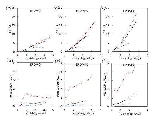
**Figure 4.** Self-heating versus strain for EPDM-0 (*a*), EPDM-40 (*b*) and EPDM-80 (*c*) during single uniaxial loading at the nominal strain rates  $10^{-2}$ .s<sup>-1</sup>(blue dotted line),  $10^{-1}$ .s<sup>-1</sup> (black continuous line), and 1.s<sup>-1</sup> (red dashed dotted line). Corresponding heat source versus strain for EPDM-0 (*d*), EPDM-40 (*e*) and EPDM-80 (*f*).
