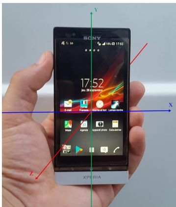
Figure 3: Coordinate system used by the Android Sensor API.
