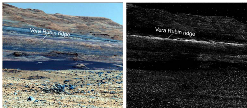
Figure 10. (left) Mastcam false color from Sol 468, product identifiers 00186400(0–6), showing VRR from several kilometers away. (right) R6 to R4 (1,013 to 900 nm) slope map showing the deep ferric absorptions (white) associated with the bedrock on VRR compared with surrounding Murray formation. After Johnson et al. (2016) and Wellington et al. (2017).
