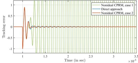
Fig. 7. Case 2 - comparison between direct approach and nonideal CPRM with  $\omega_c = 2\pi \cdot 8 \text{ rad s}^{-1}$  for case 1 ( $K_{cp}$ ) and case 2 ( $\tilde{K}$ ).
