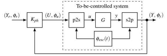
Fig. 1. Block-diagram of the phasor-based control architecture.
