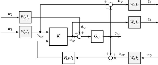
Fig. 4. Considered criterion for the  $H_\infty$  synthesis.
