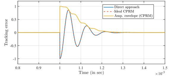
Fig. 5. Case 1 - comparison between the tracking errors of direct approach ( $G, K$ ) and ideal CPRM ( $G_{cp} K_{cp}$ ).
