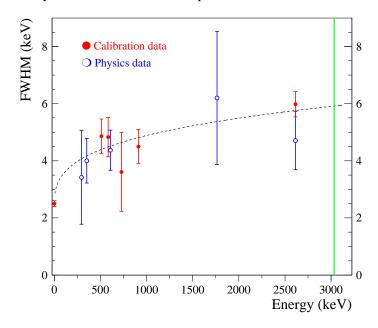
**Figure 4.** Energy dependence of the 279 g Li<sub>2</sub><sup>100</sup>MoO<sub>4</sub> bolometer energy resolution (FWHM) measured in the calibration (filled circles; 12 mK) and physics (open circles; 18 and 12 mK) runs. The fitting curve is shown by the dashed line, while the solid line indicates the <sup>100</sup>Mo  $Q_{2\beta}$ .
