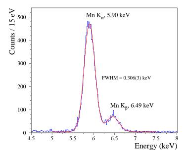
**Figure 2**. The energy spectrum of the  $^{55}$ Fe X-ray source measured by a 1.4 g Ge bolometric light detector over 913 h (12 and 18 mK data) in the CROSS pulse tube based cryogenic facility at the Canfranc underground laboratory (Spain). A fit to the data by a model assuming a double-Gaussian function and a flat background component is shown by solid (red) line. The energy resolution (FWHM) is quoted for the 5.9 keV X-ray peak of Mn  $K_{\alpha}$ .
