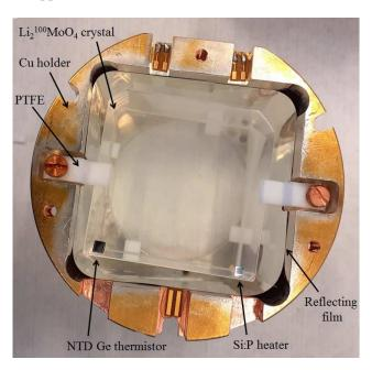
**Figure 1**. A photograph of the partially assembled  $\text{Li}_2^{100}\text{MoO}_4$  scintillating bolometer; the construction elements (see text) are labeled. A  $\oslash 45$  mm hole at the bottom of the holder, visible in transparency, acts as an entrance window for the  $\text{Li}_2^{100}\text{MoO}_4$  scintillation light to be registered by a bolometric Ge light detector.
