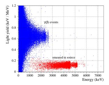
**Figure 5**. Light yield as a function of energy deposited in the LMO and measured in a 125 h long  $^{232}$ Th calibration at 12 mK. The energy scale is calibrated with  $\gamma$  quanta. The population of  $\gamma(\beta)$  events is clearly separated from the  $\alpha$  events, mainly originated by the  $^{238}$ U/ $^{234}$ U smeared  $\alpha$  source. The  $\alpha$  events shown in red were selected above 1 MeV with a LY cut below 0.25 keV/MeV.
