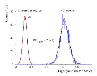
**Figure 6.** The light yield distributions for  $\alpha$  and  $\gamma(\beta)$  particles, selected in the 2.0–5.1 MeV energy interval. The former distribution is rescaled by a factor 0.1 to improve the visibility of the later one. A Gaussian fit to each distribution is shown by a solid line. The discrimination power between the two populations is  $\sim$ 8.
