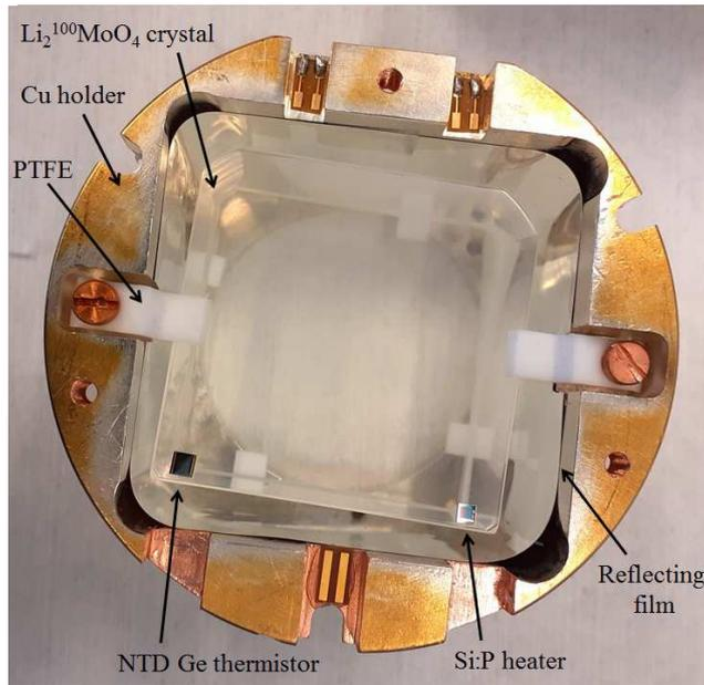
**Figure 1.** A photograph of the partially assembled  $\text{Li}_2^{100}\text{MoO}_4$  scintillating bolometer; the construction elements (see text) are labeled. A  $\varnothing 45$  mm hole at the bottom of the holder, visible in transparency, acts as an entrance window for the  $\text{Li}_2^{100}\text{MoO}_4$  scintillation light to be registered by a bolometric Ge light detector.
