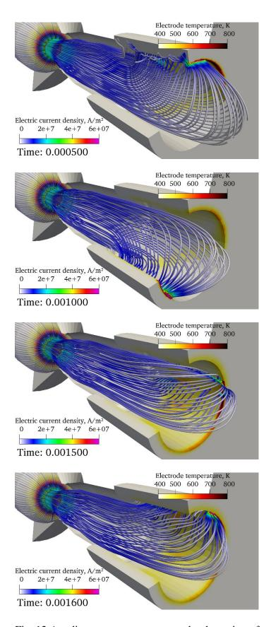
Fig. 12 Anodic arc root movement under the action of an external axial magnetic field of 0.05 T. Frequency of arc displacement: 800 Hz
