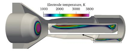
Fig. 9 Temperature of the electrodes with the anode inner surface zoomed in. Nozzle  $\emptyset = 9$  mm, 500 A, 60 NLPM Ar. Straight gas injection, no external magnetic field.
