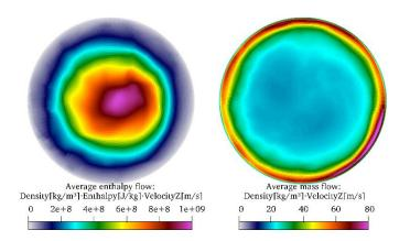
Fig. 17 Enthalpy flow rate and mass flow rate for an external magnetic field of 0.05 T. Predicted total enthalpy flow rate: 23.7 kJ/s and total mass flow rate: 1.77.10<sup>-3</sup> kg/s in the anode exit plane
