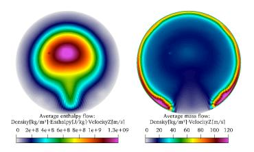
Fig. 10 Enthalpy flow rate and mass flow rate at the nozzle exit. Nozzle  $\emptyset = 9$  mm, 500 A, 60 NLPM Ar. Straight gas injection, no external magnetic field.
