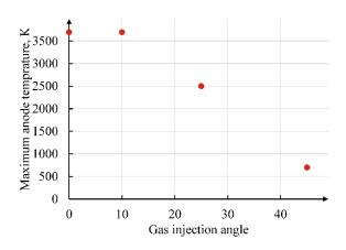
Fig. 8 Variation of the maximum anode temperature with the plasma-forming gas injection angle (no external magnetic field)
