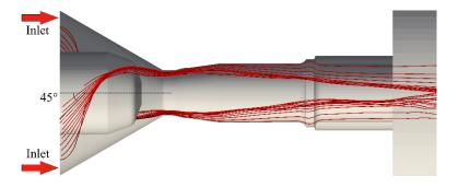
Fig. 6 Gas velocity streamlines with a plasma-forming gas injection angle of  $45^{\circ}$  and no external magnetic field
