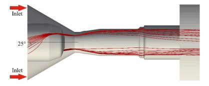
Fig. 5 Gas velocity streamlines with a plasma-forming gas injection angle of  $25^\circ$  and no external magnetic field
