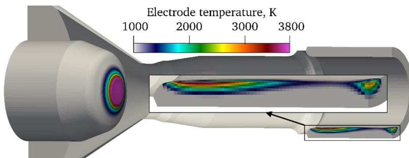
Fig. 9 Temperature of the electrodes with the anode inner surface zoomed in. Nozzle  $\text{\O} = 9$  mm, 500 A, 60 NLPM Ar. Straight gas injection, no external magnetic field.
