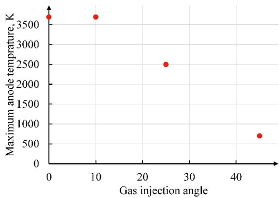
Fig. 8 Variation of the maximum anode temperature with the plasma-forming gas injection angle (no external magnetic field)
