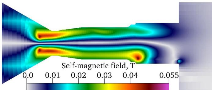
Fig. 11 Self-magnetic field generated by the arc current
