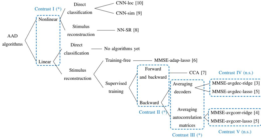
Figure 3: The included AAD algorithms in this comparative study and the planned contrasts in the statistical analysis. (\*) indicates a significant difference ( $p < 0.05$ ), (n.s.) indicates a non-significant difference.
