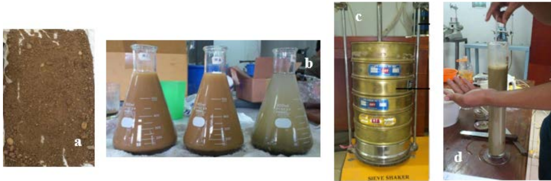
Figure 4. Sediment laboratory test: a) air-dried sediment, b) specific gravity test, c) sieve analysis, and d) hydrometer test
