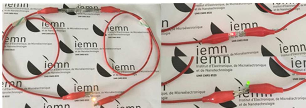
**Figure 8:** Photographs of LEDs (yellow, red and green) powered by two asymmetric supercapacitors connected in series.
