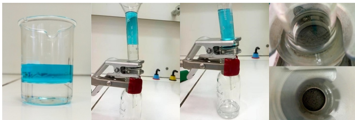
Figure 12. Photographs of the chloroform/water separation process ( video S2 ). The water was dyed with Methylene Blue for clear observation.
