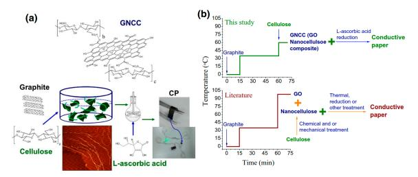
**Figure 12.** (a) A schematic flow diagram illustrates CNC/GO (GNCC) production using the one-pot method and further reduced to form conductive paper (CP, CNC/RGO). (b) A comparison of the present one-pot process with the conventional approach in literature. Reproduced with permission from Reference [177]. Copyright ©2019, Springer.
