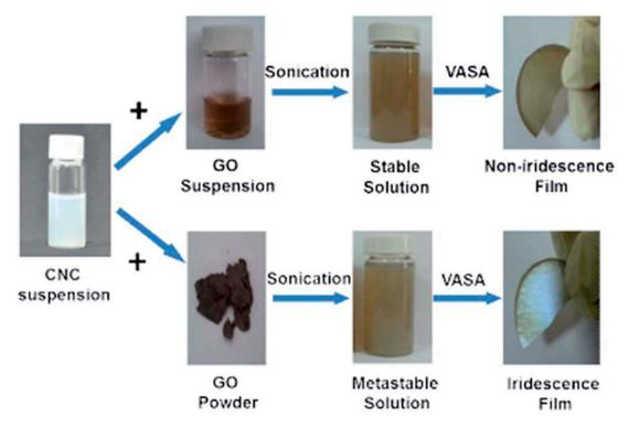
**Figure 7.** Schematic illustration of the preparation process of GO/CNC hybrid films with or without iridescence. Reproduced with permission from Reference [151]. Copyright ©2014, The Royal Society of Chemistry.
