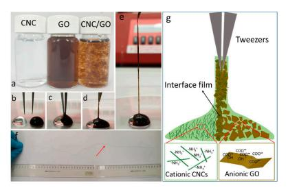
**Figure 14.** (a) suspensions of cationic CNC and GO and a dual precipitated complex after simple mixing; (b–e) CNC/GO hybrid filament drawing process; (f) a single dried CNC/GO hybrid filament with a diameter of ~33  $\mu$ m and a length of 53 cm; (g) a scheme illustrating the CNC/GO hybrid filament drawing process. Reproduced with permission from Reference [178]. Licensed under a Creative Commons Attribution 3.0 International License (https://creativecommons.org/licenses/by/3.0/).
