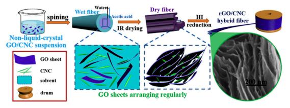
**Figure 13.** Schematic illustration of the preparation of CNC/RGO hybrid fiber. Reproduced with permission from Reference [130]. Copyright ©2018, Elsevier.
