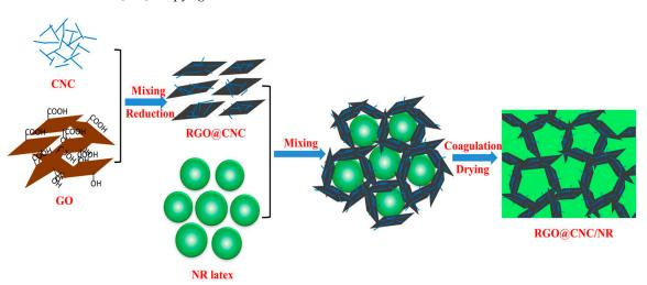
**Figure 16.** Schematic presentation of the synthesis of CNC/RGO/NR nanocomposite. Reproduced with permission from Reference [182]. Copyright ©2016, Elsevier.
