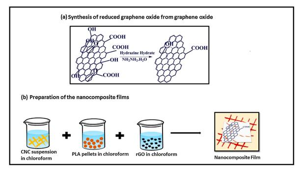
**Figure 17.** Schematic illustration of (**a**) the synthesis of reduced graphene oxide (RGO) from GO, (**b**) the method employed to prepare nanocomposite films. Reproduced with permission from Reference [185]. Copyright ©2017, Elsevier.
