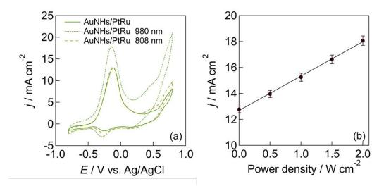
**Figure 3. Electrocatalytic methanol oxidation under light irradiation**. (a) Cyclic voltammograms of AuNHs/PtRu in 0.1 M NaOH / 0.1 M CH<sub>3</sub>OH upon light irradiation at 980 and 808 nm at 2 W/cn<sup>2</sup>. (b) Influence of 980 nm laser light power density on the current density of AuNHs/PtRu in 0.1 M NaOH / 0.1 M CH<sub>3</sub>OH.
