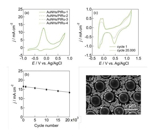
Figure 5. Interface characteristics. (a) CV curves of 4 AuNHs/PtRu interfaces in 0.1 M NaOH / 0.1 M CH<sub>3</sub>OH at a scan rate of 20 mV/s in dark. (b) Variation of methanol oxidation current under 980 nm (2 W/cm<sup>2</sup>) light illumination over 20.000 cycles. (c) Cyclic
