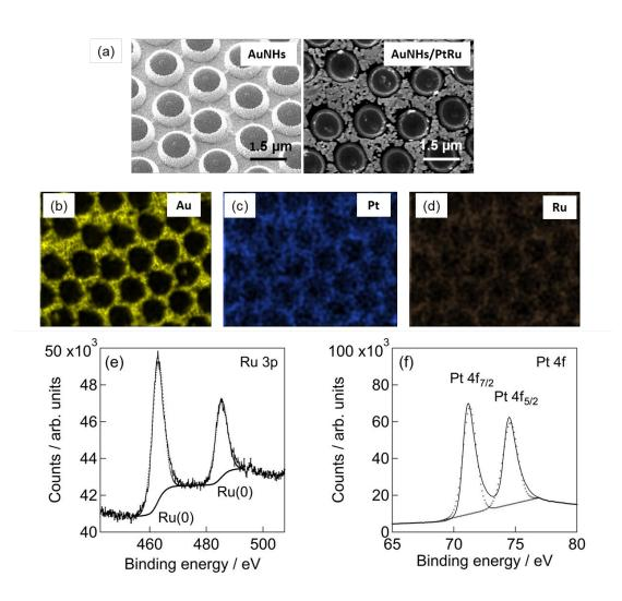
**Figure 2.** Physico-chemical features of AuNHs/PtRu electrodes. (a) SEM images of AuNHs and AuNHs/PtRu. (b-d) EDS mapping of Au (b), Pt (c) and Ru (d) of the AuNHs/PtRu electrode. (e) Core level spectra of Ru 3p. (f) Core level spectrum of Pt 4f.
