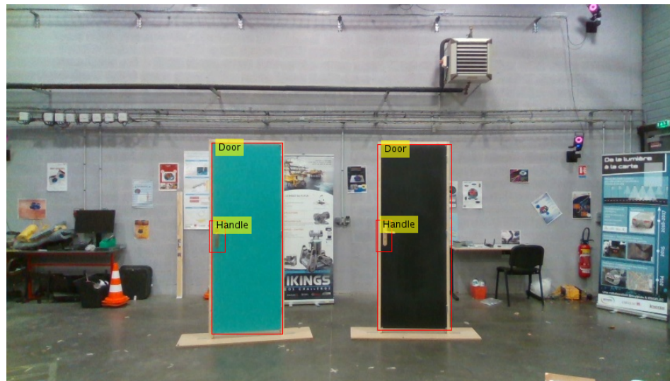
Figure 6. Arrangement of doors in the validation dataset. The ground truth bounding boxes are displayed in red with the associated label overlaid in yellow. In the top-right of figure, we can see a part of the Vicon motion capture system within cameras network.
