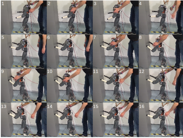
Fig. 8: Frames 1 to 6 show the reaction to a push. COMAN moves its arms towards the configuration computed from the optimization step. Frames 7 to 11 show the compliant behavior in case of an equally distributed push when COMAN is in contact with the environment. Frames 12 to 16 shows the same behavior in case of a non-equally distributed push.
