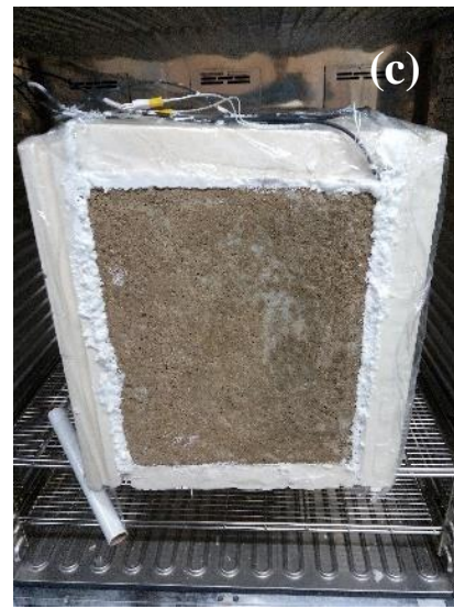
Figure 2: a) Overall experimental setup, b) humidity/temperature sensors after installation in the wall cross-section, c) Picture of the wall connected to the passive cell (indoor environment) and installed inside the HPP750 climatic chamber (outdoor environment).
