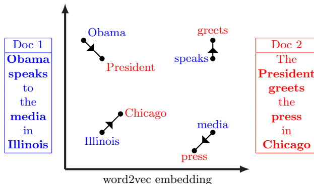
Fig. 2. An illustration of the Word Mover’s Distance by [19]. The distance between the two documents is given by the minimum cumulative distance that all the words in Doc 1 need to travel in order to reach the words of Doc 2.
