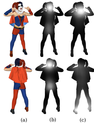
Fig. 3. Illustration of 6 partial point clouds, each line represents: (a) the rendered view, (b) the ground-truth saliency information and (c) the resulted saliency based on interpolation technique.
