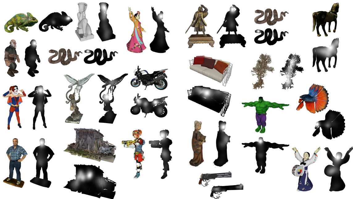
Fig. 2. Illustration of one view of the 3D graphic contents and its corresponding saliency collected from human fixations; also called saliency ground-truth.
