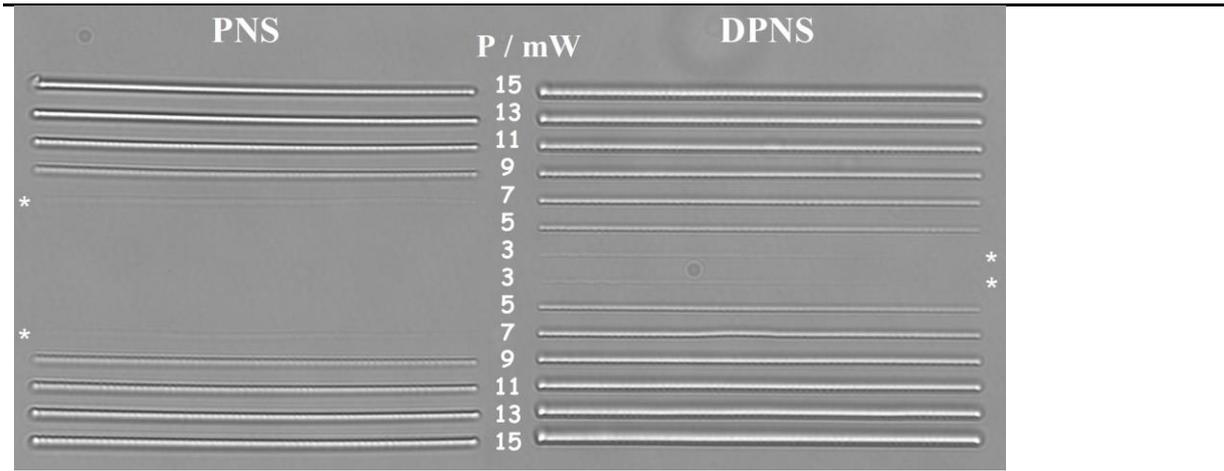
**Figure 7.** Two-photon polymerized lines fabricated for distinctive laser excitation powers ( $\lambda_{ex} = 780 \text{ nm}$ ,  $\tau_{exp} = 2 \text{ ms}$ ). The star pictogram indicates the corresponding value of  $P_{th}$  at 780 nm. Formulations: Poly(ethylene glycol) diacrylate mixed with **MDEA** (wt 5 %) and with : **PNS** (0.35 wt %  $\leftrightarrow$  13.6 mM) and **DPNS** (0.4 wt %  $\leftrightarrow$  6.8 mM).
