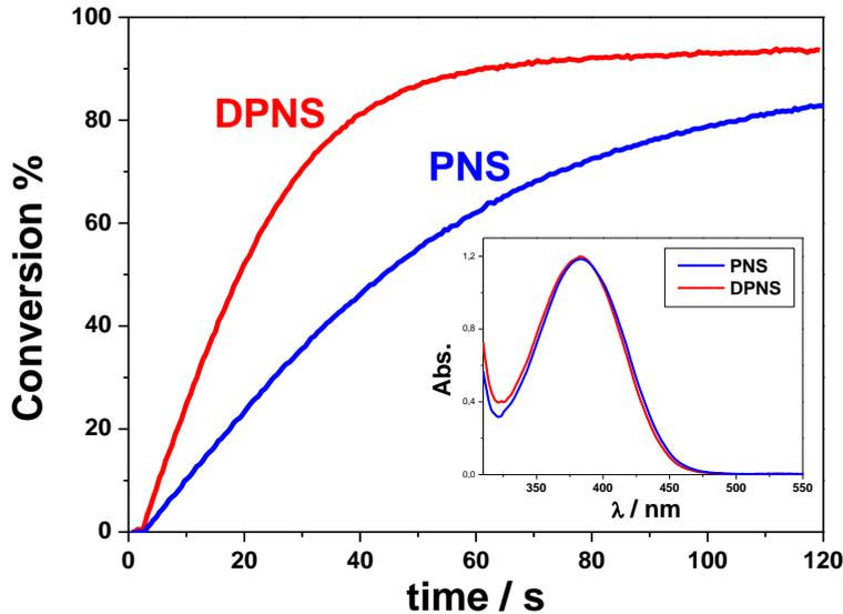
**Figure 5.** Real-time FTIR kinetics of C=C bonds conversion curves upon irradiation of diacrylate formulations ( $I_{365\text{nm}} = 5 \text{ mW cm}^{-2}$ ). Photoinitiating systems: **PNS / MDEA** (0.35 wt % / 5 wt %) and **DPNS / MDEA** (0.4 wt % / 5 wt %). Inset: Absorption spectra of the corresponding resins (30  $\mu\text{m}$ -thick-films).
