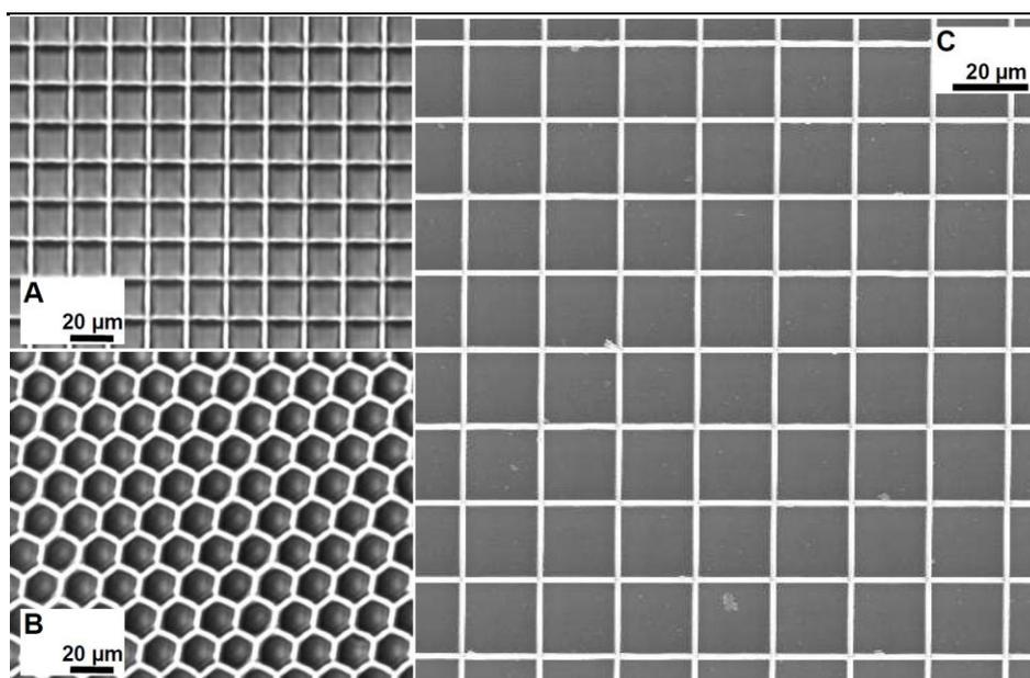
**Figure 8.** A-B Transmitted light microscope images of periodic 2D  $\mu$ -structures. Formulation: diacrylate resin with **DPNS** / **MDEA** (0.4 wt % / 5 wt %). ( $\lambda_{\text{ex}}$  : 780 nm, P = 5 mW,  $\tau_{\text{exp}}$  = 2 ms). C. SEM images of  $\mu$ -grid. Formulation: **PETIA** with **DPNS** / **MDEA** (0.4 wt % / 5 wt %). ( $\lambda_{\text{ex}}$  : 780 nm, P = 5 mW,  $\tau_{\text{exp}}$  = 2 ms).
