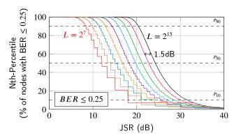
Figure 7: Percentiles for nodes with predicted  $BER \le 0.25$  as a function of an insider smart jammer power JSR, for different spreading sequences (SS) lengths  $L \in \{2^7, 2^8, ..., 2^{15}\}$ .
