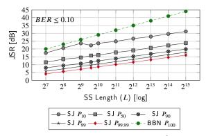
Figure 8: Percentiles of nodes with  $BER \le 0.1$  for a Jammer with power JSR (dB), as a function of the SS length L.
