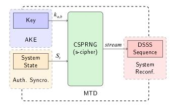
Figure 2: MTD Proposal: Cryptographically Secure PR-DSSS.
