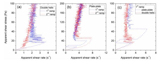
Fig. 2. Effect of the flow history on the shape of experimental flow curves of the isotropic shape particle (CC) suspensions at CC particle volume fraction  $\varphi_p$ =0.68 measured in mixer type (a) and plate-plate (b) geometries. All the reported flow curves correspond to the ascending branch of either the 1<sup>st</sup> or the 2<sup>nd</sup> stress ramp. Flow curves obtained during the 1<sup>st</sup> ramp in both rheometric geometries are compared in figure (c).
