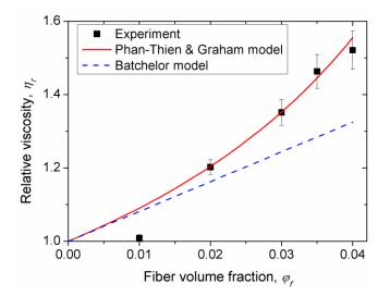
Fig. 9. Relative viscosity  $\eta_r$  of the suspension of PA fibers dispersed in a Newtonian solvent (glycerin) as function of the fiber volume fraction  $\varphi_f$ . Points correspond to the experiment using in the mixer type geometry, solid lines to the predictions of Phan-Thien & Graham model [Eq. (A-7)] and Batchelor model.
