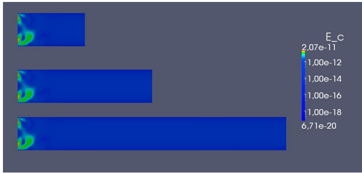
Figure 7: Snapshot of Kinetic energy for A = 4, 8, 16 at time t \simeq 17s .
