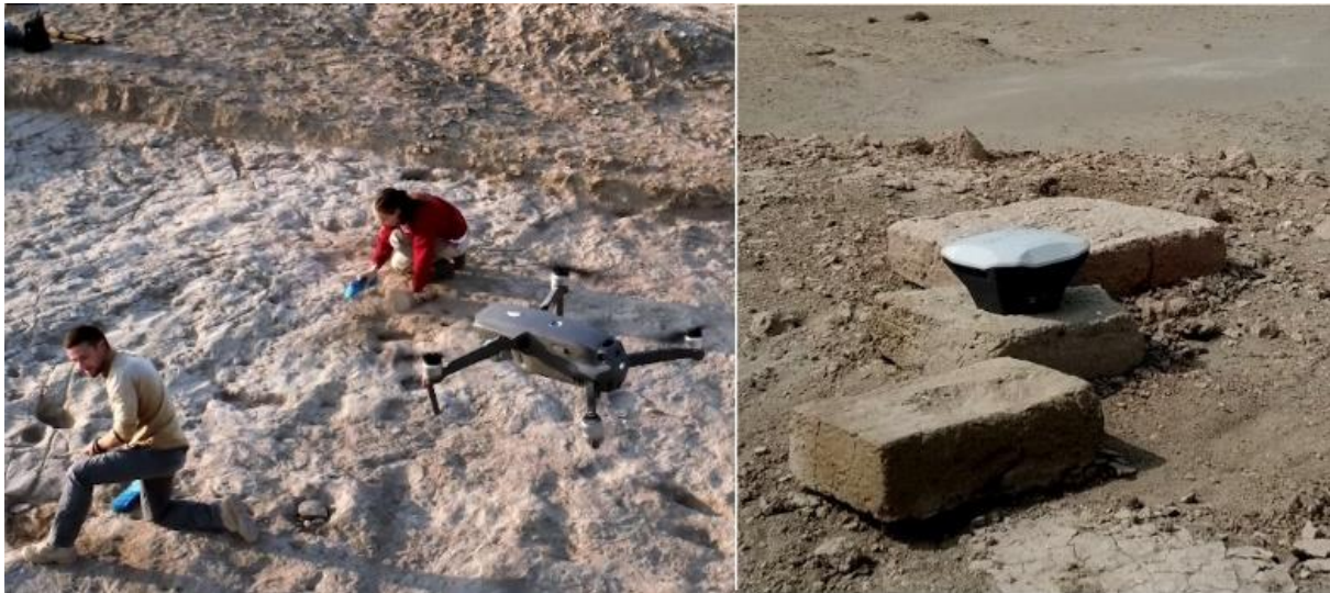
Fig. 1 – Left: the Mavic Air 2 pro drone flying above the ‘Uwaili excavation sector, Right: a ground control point made up of bricks and measured with the Emlid Reach RS+ GPS.
