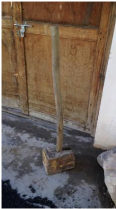
Rammer in wood for rammed earth construction (Ladakh, India)
