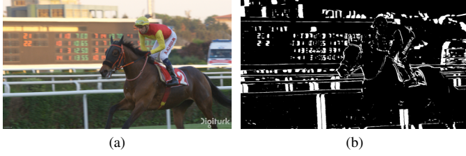
Fig. 4. Example of thresholded motion difference with (a) the original image of the Jokey sequence and (b) the thresholding activation map with threshold Th = 25 .
